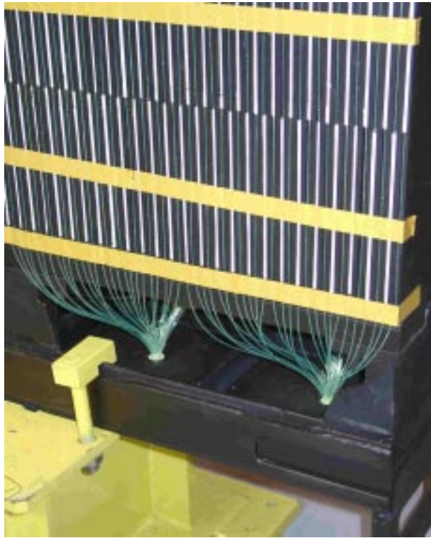
Fig.13. The fiber routing in bundles.
