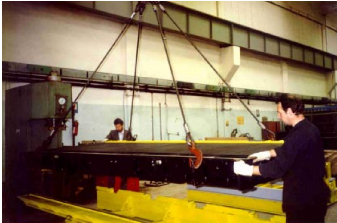
Fig.8. Installing the Module-0 on to the transport tool for the check in the IHEP workshop.
