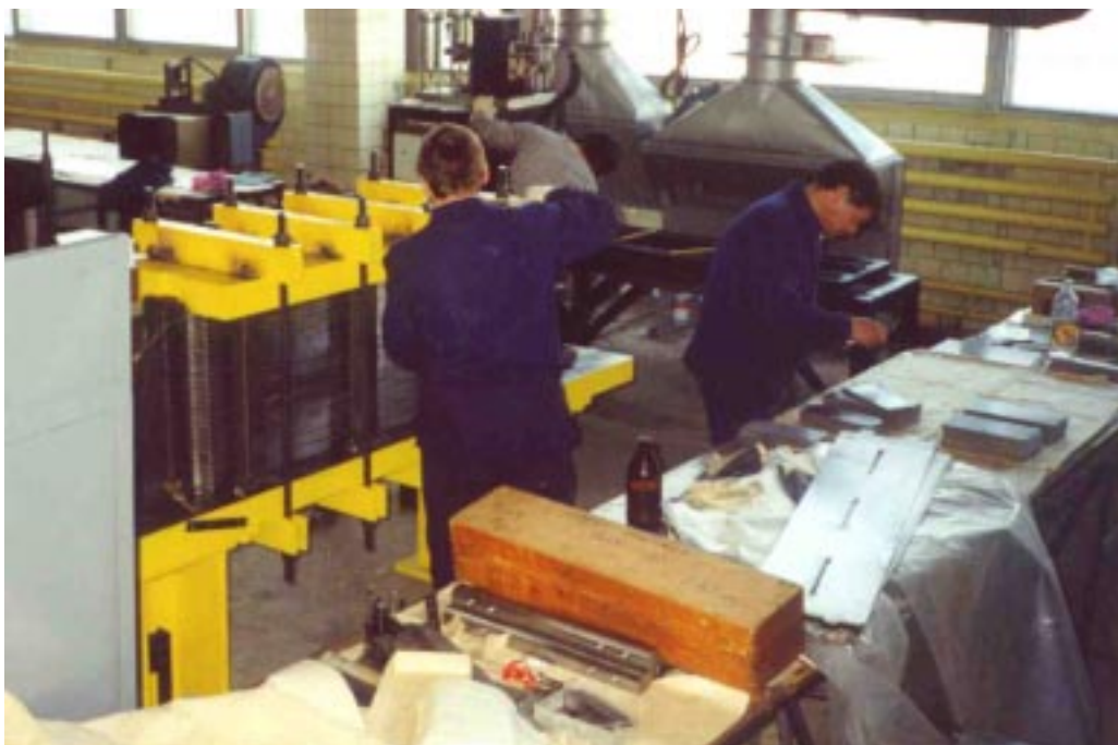
Fig.2. The sub-module assembly area in the IHEP workshop. The gluing tool seen on the left. The gluing automatic machine seen on the back covered by the air exhaust.
